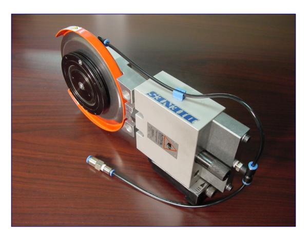
Many high quality steel knife blades with various cutting edge bevels and angles can be employed to maximize knife life and roll edge quality.
